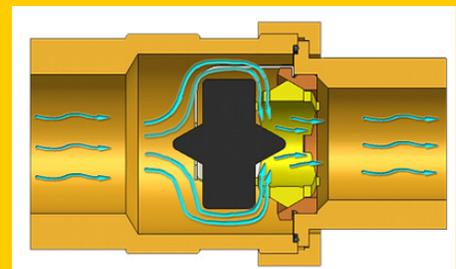
Increased pressure forces the diaphragm to push against the orifice, which results in limited flow. The greater the pressure, the more the diaphragm closes the orifice space available. This is why the Mesurflo® adapts to pressure increases.
