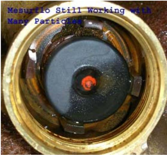
Mesurflo technology does very well with small particulates. The iron filings accumulate in the low velocity area around the base of the Mesurflo. As long as the opening between the orifice and diaphragm is large enough these particles pass through during the low pressure portion of the test, freeing the valve from contamination. A picture of the Mesurflo after the test at 0.8 oz/hr is provided to the left. The Mesurflo was still controlling flow!
